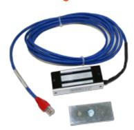
This small electromagnetic door lock with holding force of 700 N, which corresponds to 70 kg, is suitable for racks which cannot be fitted with a CONTEG electronic handle. LED indicates the status of the lock: unlocked, locked, open or breach. Powered from the main unit.
