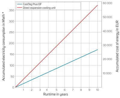
\* The unit's consumption is dependent on its location, or rather, the annual course of temperature at the location. The unit's consumption over the course of the year and use ratio of the individual cooling modes were calculated using nominal values and the annual course of temperature in Prague.
