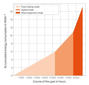
\* The unit's consumption is dependent on its location, or rather, the annual course of temperature at the location. The unit's consumption over the course of the year and use ratio of the individual cooling modes were calculated using nominal values and the annual course of temperature in Prague.
